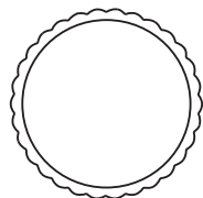
11671 Serrated Round Tube Size. 3 X .125 Length. Ft. 24 Wt. Lin Ft. 1.913
