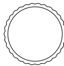
14045 Serrated Awning Tube Size: 7/8 X .044 Lgth. Ft. 24 Wt. Lin. Ft.: .138 .
