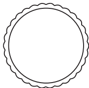
11671 Serrated Round Tube Size 3 x .125 Lgth. Ft. 24 Wt. Lin Ft. 1.913
